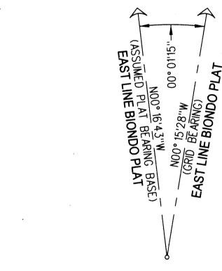
TO CONVERT ASSUMED PLAT BEARINGS TO STATE PLANE GRID BEARINGS ROTATE PLAT BEARINGS 00° 01'15" CLOCKWISE
